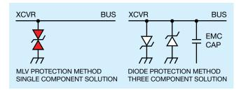
Figure 1. Comparison of past node protection methods to MLV node protection methods.
