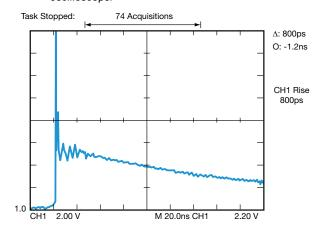
The open circuit response of the ESD test fixture with a 9kV ESD pulse is shown in Figure 3.
