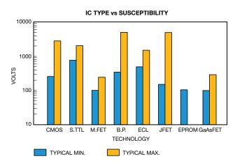
Figure 3. IC Type E Field Susceptibility
