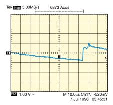
Fig. 6. 12 V Relay Transient without protection 105 V 50 V/Division
