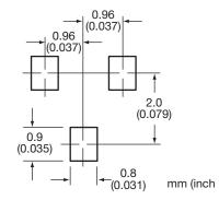
Figure 1B. SOT23- Solder Pad Layout
