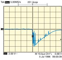
Fig. 2. Geared Motor Running noise without protection 12 V pk-pk 2 V/ Division
