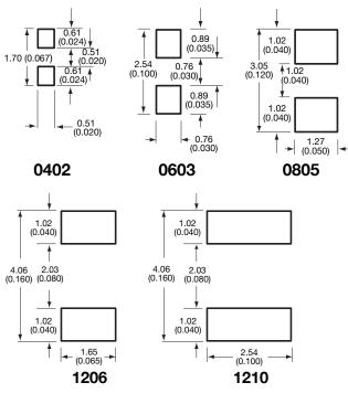
Figure 1: TransGuard® Solder Pad Dimensions
