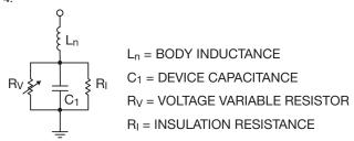
Figure 4. Antenna Varistor
