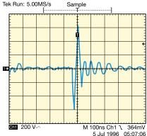
A x10 probe was connected to the scope and one leg of the relay/motor coil; the probe's ground was connected to the other relay coil/motor wire. The scope was triggered on the pulse and waveforms printed.
