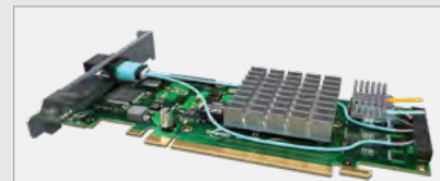
PCIe®-over-Fiber adaptor card (PCOA) supports transparent and non-transparent bridge links using PCUO FireFly™
