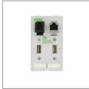
RJ45; RJ12; USB; USB (type A) 1 × RJ45, 8-pole. Metal, CAT5e (socket/socket) 1 × RJ12, 6-pole. Plastic 2 × USB (socket/socket) type A Order No. 20.90 10 55
