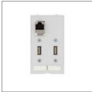
RJ45; USB; USB (type A) 1 × RJ45, 8-pole. metal, CAT5e (socket/socket) 2 × USB (socket/socket) Type A Order No. 20.90 10 59
