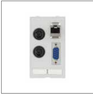
RJ45; SUB-D9; PS2; PS2 1 x RJ45, 8-pole. Metal, CAT5e (socket/socket) 1 x SUB-D9 (pin/pin) 2 x PS2 (6-pole. solder connection) Order No. 20.90 10 78
