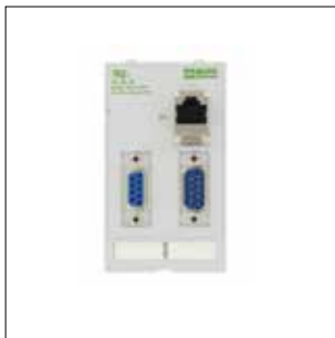
RJ45; SUB-D9; SUB-D9 1 × RJ45, 8-pole. metal, CAT5e (socket/socket) 1 × SUB-D9 (socket/socket) 1 × SUB-D9 (pin/pin) Order No. 20.90 10 62
