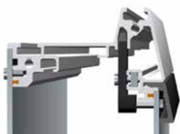
Front panel installation screwed from front
