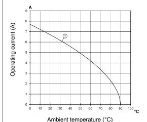
① Conductor cross-section 0.52 mm²
