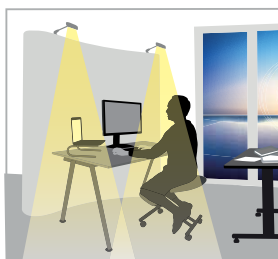
Model 18.51 automatically switches the lights on when the light level is low and movement is detected.
