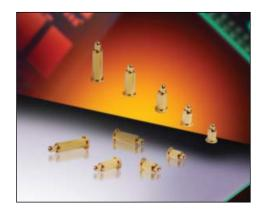
Single Pogo Pin contacts provide high cycle life in industrial and medical applications where reliability and robustness is critical. Pogo Pins provide 10,000 mating cycles and are ideal in pluggable module applications where the end customer has to handle a product daily. Pogo Pins are designed to mate with gold plated PCB pads or flat contacts in docking/cradle applications to function as the charging, data transfer or programming interface to a portable device.
