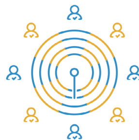
Active Antennas Eliminate nulls by "steering" the emission in real-time by using intelligent algorithms and flexible antenna structure
